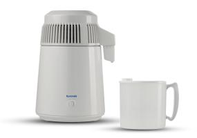
Water distiller for obtaining distilled water by boiling and subsequent steam condensation. It distils 0.7 L of water per hour. 4-litre capacity. It fulfils the safety and electromagnetic compatibility (2014/30/EU) and low voltage (2014/35/EU) tests.
