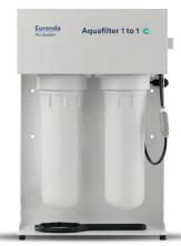
Device for the production of deionised water for autoclaves, in accordance with EN 13060 (<15  $\mu$ S/cm). Only one Euronda Pro System autoclave can be supplied. It deionises on average 1 litre of water per minute. It can be equipped with automatic shut-off device. It can be placed directly on the worktop or inside a cabinet, as well as mounted to a wall. Included in the initial equipment are two ion exchange resins.
